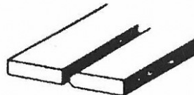
DOUBLE BEVEL JOINT
