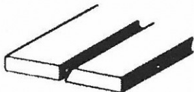
SINGLE BEVEL JOINT
