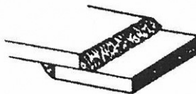
DOUBLE FILLET LAP JOINT
